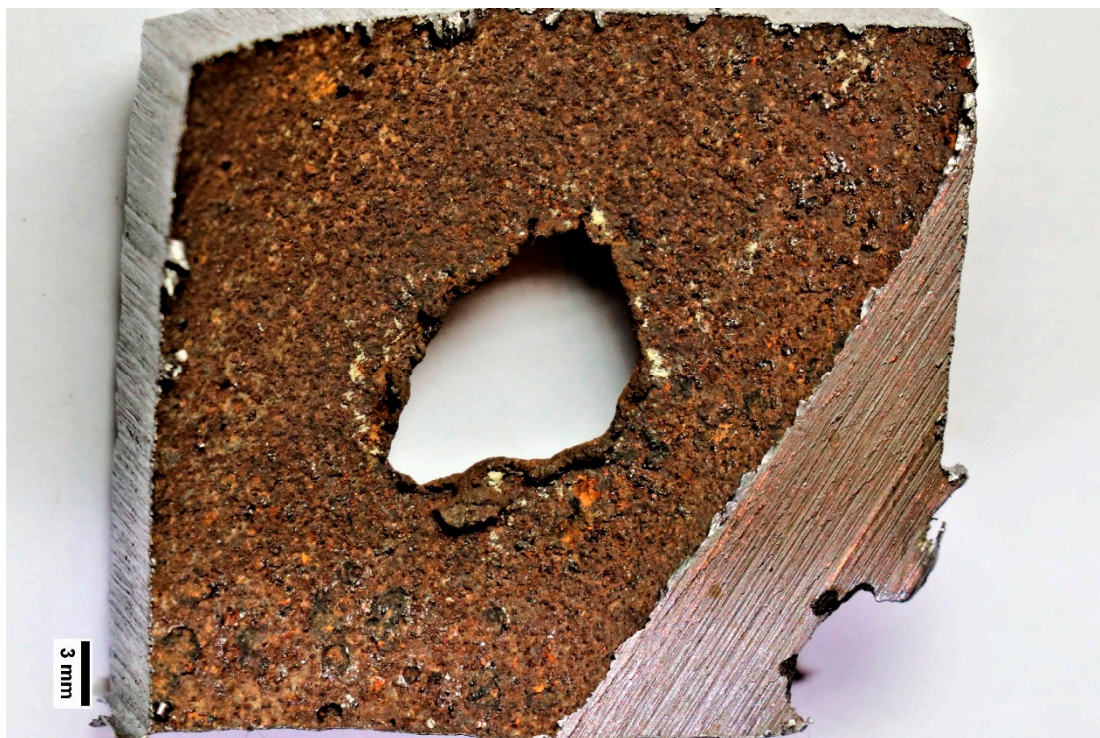
Figure 3. An inner surface of the failed elbows.
