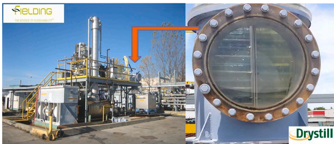
Fig. 3. Pass-through distillation pilot-scale unit in operation at Fielding Chemical Technologies, where the stripping-absorption module built by Drystill plays a key role [8].
