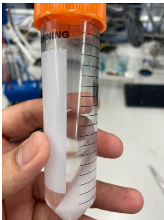
Figure 4.12: ChCl:AMP (1:6) solvent with precipitate after reacting with CO_2
