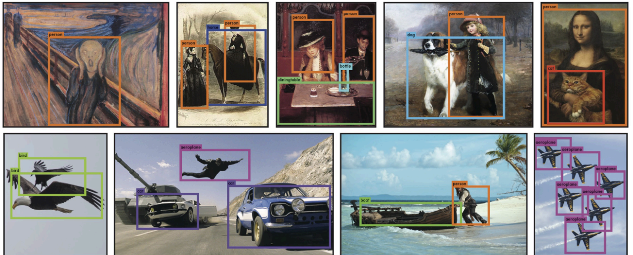
Figure 2.3: From the original YOLO paper [22]. The YOLO object detector runs on simple artwork and images from the internet. There is one error in classification, the second image from the bottom row classifies a person as an airplane.
