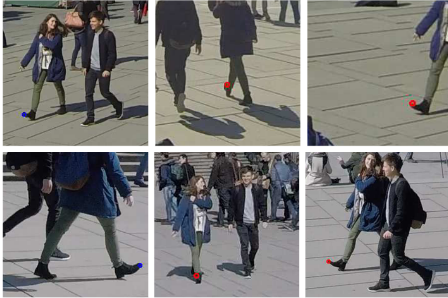
Figure 1.1: The public dataset WildTrack [6] is shown here with its calibration precision visualized. The two images on the left display the initialization points depicted in blue. These two points are projected to a single 3D point using the camera calibration information and triangulation. The four images on the right show the same object (the nose of a shoe) but from varying viewing angles. When the 3D point is back-projected to 2D pixel coordinates (using the camera calibration information of that camera angle) it shows the 2D point on the same object, only in other viewing angles. These back-projected points are shown in red.
