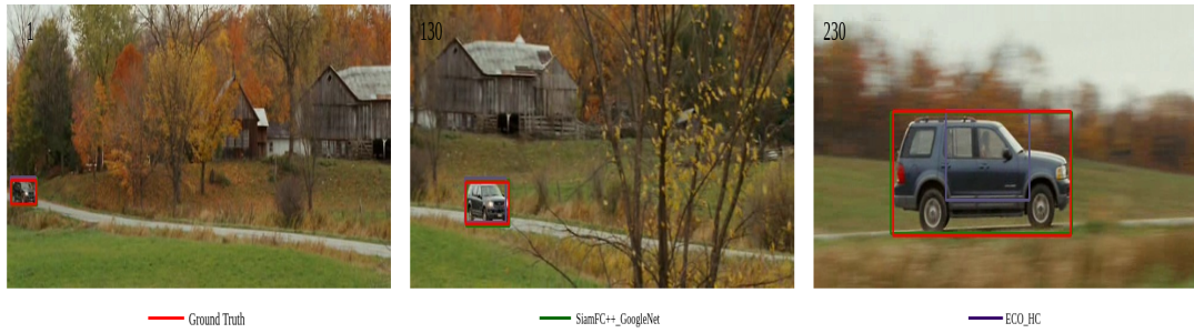
Figure 1.2: Scale Variation: the ratio of the bounding boxes of the first frame and the current frame is out of the range 2.
