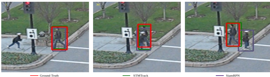
Figure 1.1: Occlusion: the target is partially or fully occluded. The top-left number is the frame step of the sequence.
