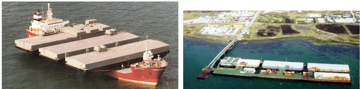
Figure B.2: The transport of the barges (left) used for the final construction of a floating seaport in Falklands (right) (Think Defence, 2015)
