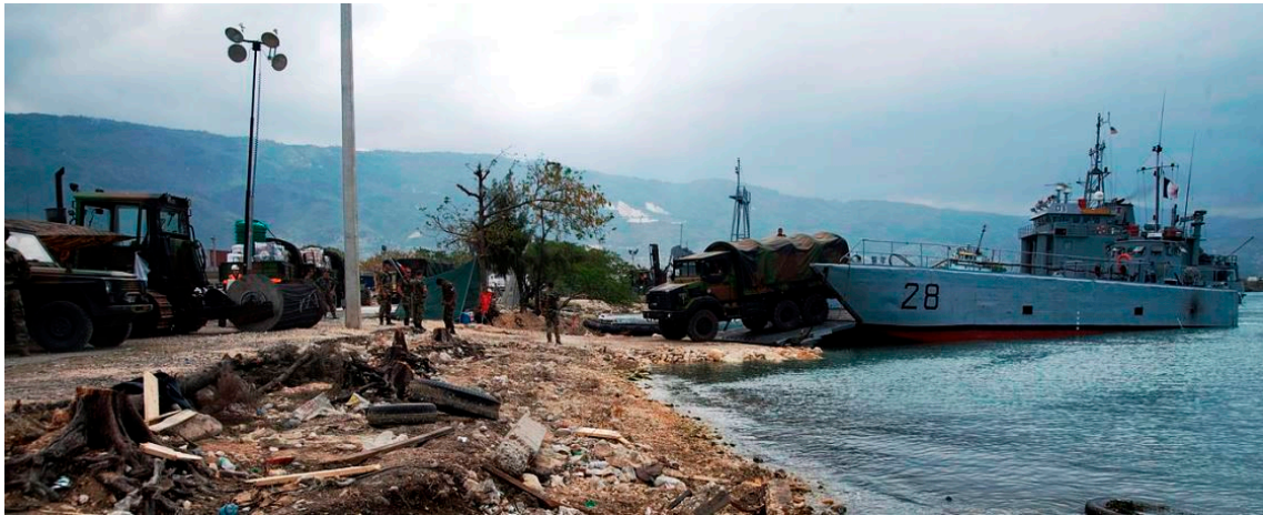
Figure B.1: Smaller ships with bow ramps, normally used by military to transfer goods from ships to shore (Think Defence, 2015)
