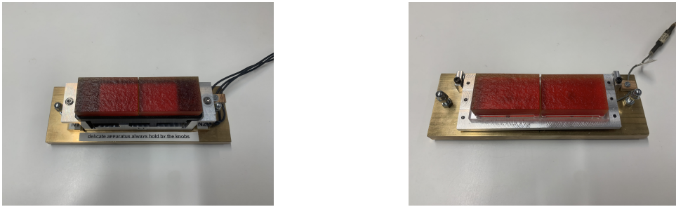
Figure 4.3. Left side: Dynamics tribometer used for roughness discrimination. Right side: Load sensor used for softness discrimination. Each containing two stimuli as used in the experiment.
