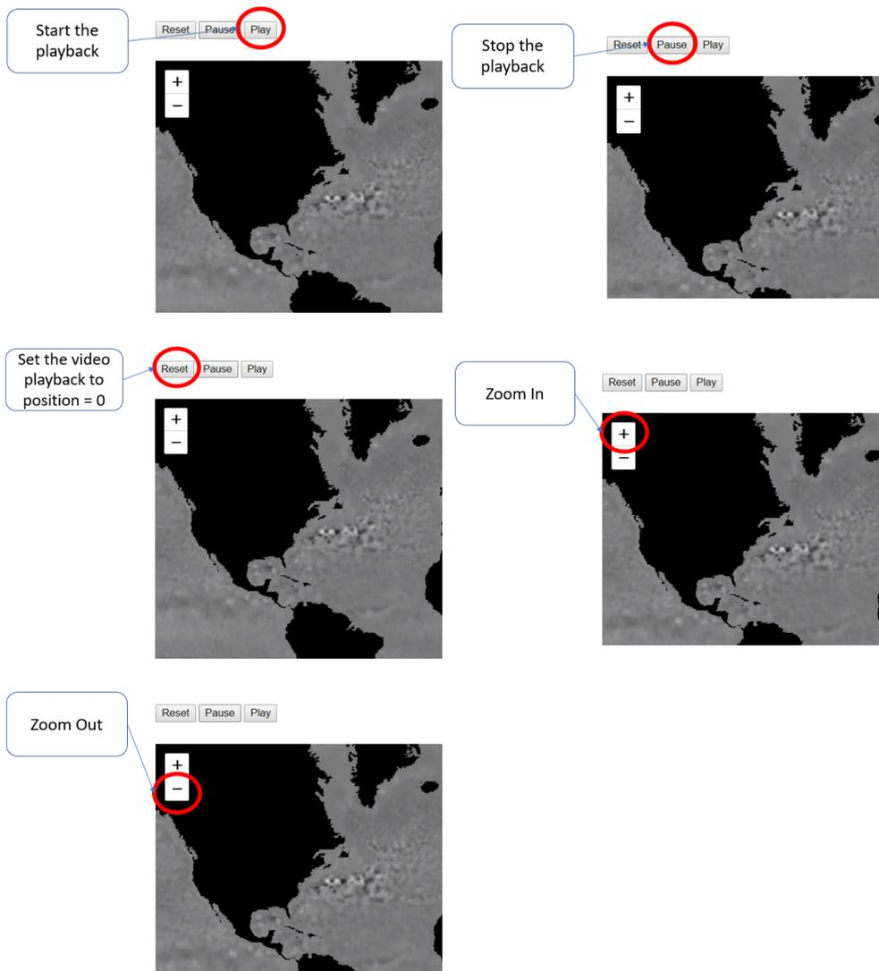
Figure 5.6: The interface of the application with the videos synchronized (zoom level 1).
