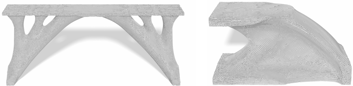
Fig. 14: Optimized lattice structures composed of 462k struts (bridge) and 351k struts (cantilever).
