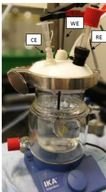
Figure A.1: Experimental setup with with the single compartment electrochemical cell, the working electrode indicated as WE, the reference electrode as RE and the counter electrode as CE; electrolyte buffer of 0.5M boric acid at a pH of 9.2.
