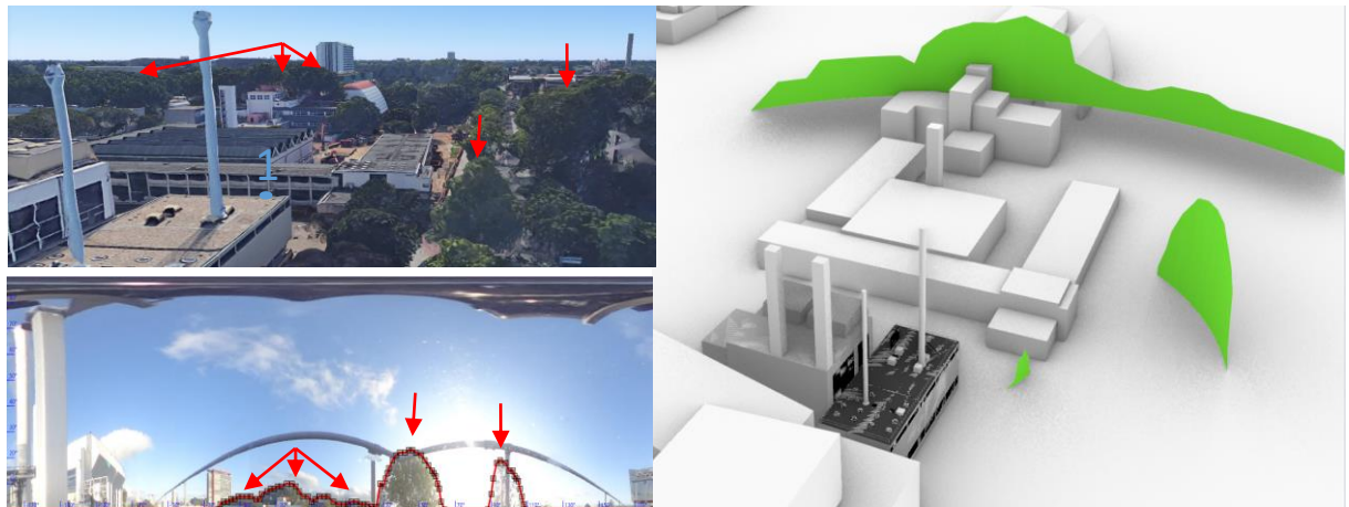
Figure 5.5: Figure displaying the process of drawing the necessary trees into the CAD design. First identifying the trees. Next drawing the tree silhouettes. And finally drawing the trees in the CAD.
