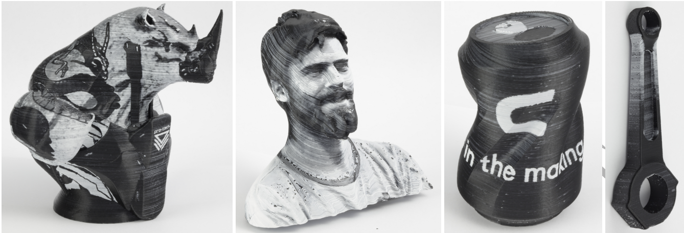
Fig. 1: 3D prints obtained by applying hatching on a 14 cm 3D portrait, a 15 cm artistic figurine, a full size soda can with textual information, and the result of a stress analysis performed on a 16 cm connecting rod of a piston engine.
