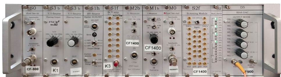
Figure 3.5: (a) Photograph of a matrix module with 48 separate channels. Each channel has a toggle switch to ground, float or connect the line. (b) Photograph of a full IVVI rack. The S0 module (far left position) contains isolated input ports, next to that are S3b modules for voltage/current bias, M2b and M1h are voltage and current measure modules respectively.
