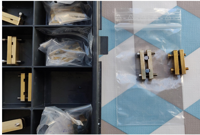
Figure 3.9: Two cylindrical samples held in custom sample holder used for grinding and polishing.
