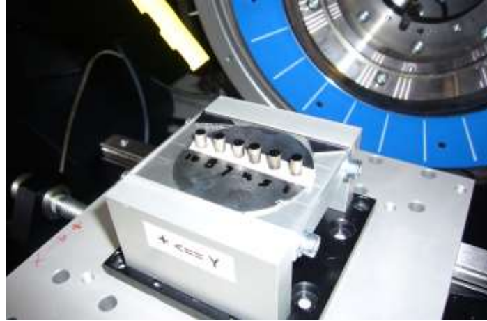
Figure 3.12: Cylindrical samples with polished top surface fixed on a Si510 wafer in a standard sample holder.
