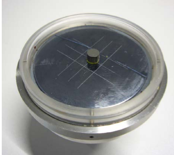
Figure 3.13: Cylindrical samples mounted on SD52 holder using plasticine.
