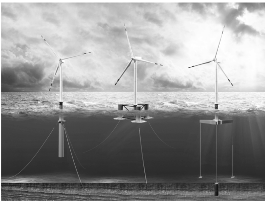
Fig. 1. Floating offshore wind turbines with a support structure in spar-buoy (left), semi-submersible (middle) and tension leg platform (right) configuration [6].
