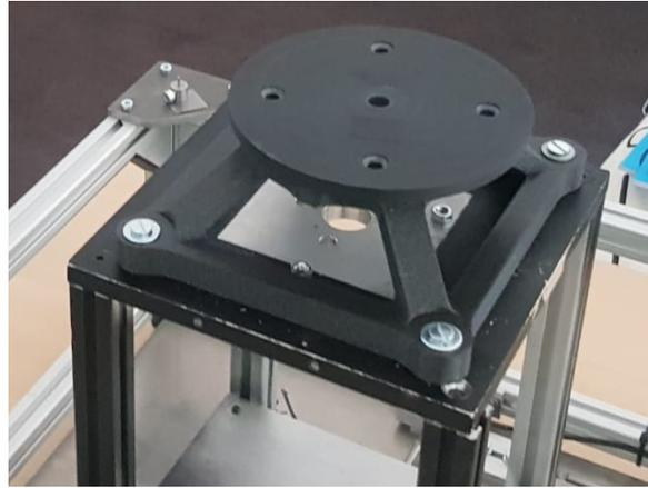
**Figure 4.5:** Attachment connecting cylinders to the balance.
