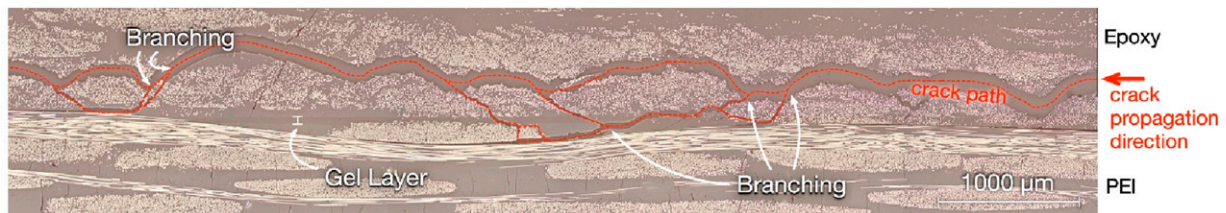
Figure 16. An optical micrograph of cracking in a failed IC20 Double Cantilever Beam specimen.
