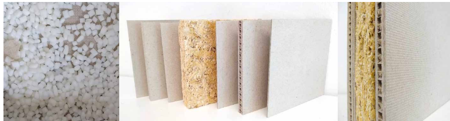
FIG. 7.12 Niaga polyester-resin pellets (left), and a basic NEP/Mycelium configuration (centre and right)
