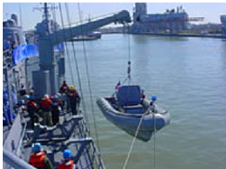
Figure 2.7: Single point crane system with tag line from bow [McTaggart et al., 2016]
