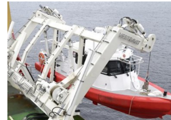
Figure 2.9: Dual lift point davit [McTaggart et al., 2016]
