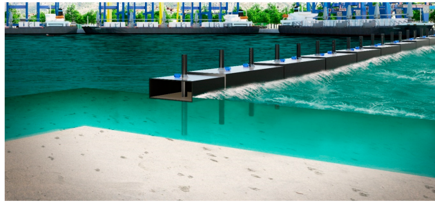
Figure 5.2: Floating breakwater [Zhao et al., 2019]
