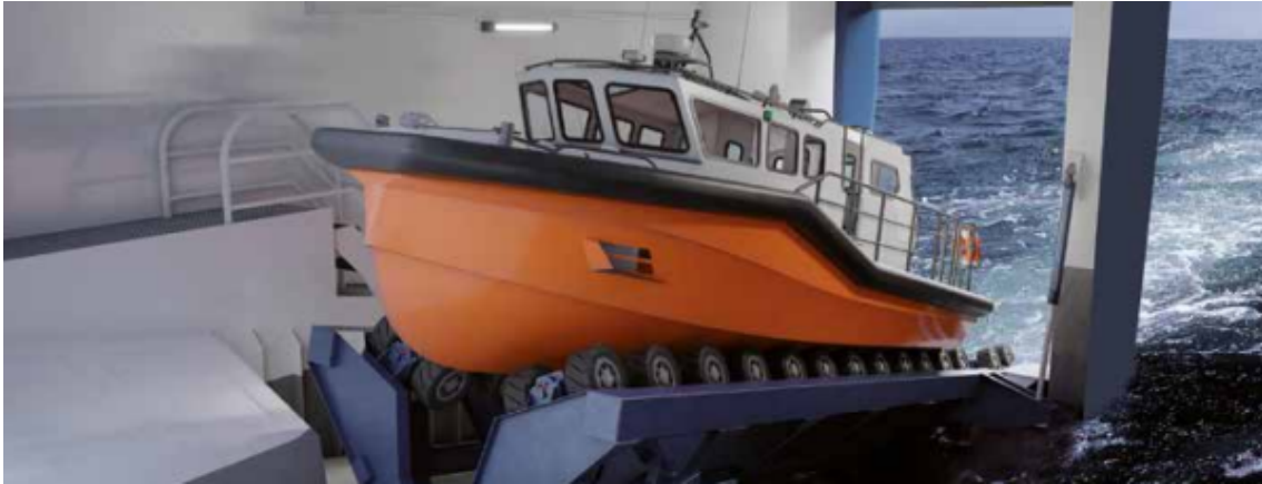
Figure 5.11: PQBS-T stern ramp system from Palfinger [Palfinger, 2022]
