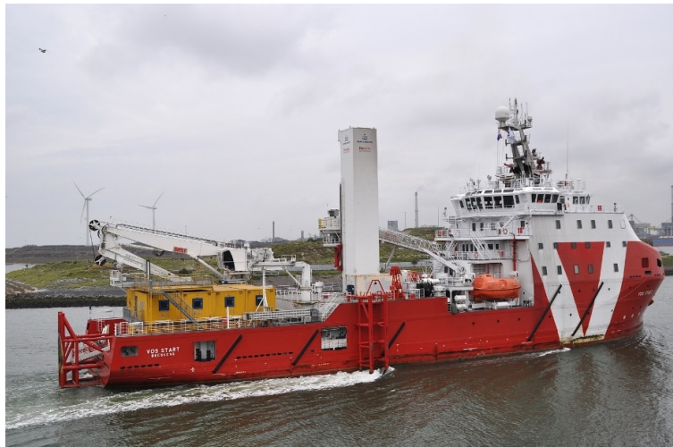
Figure 5.17: SOV with boat landing installed at the stern and starboard [Maritime, 2019]
