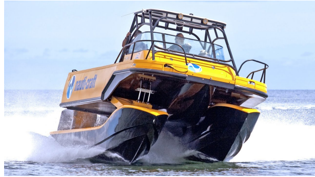
Figure 5.5: A suspension hull during a high speed turn [Craft, 2022]
