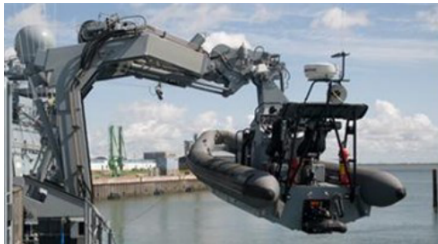
Figure 2.8: Sophisticated single point davit, restricting yaw [McTaggart et al., 2016]
