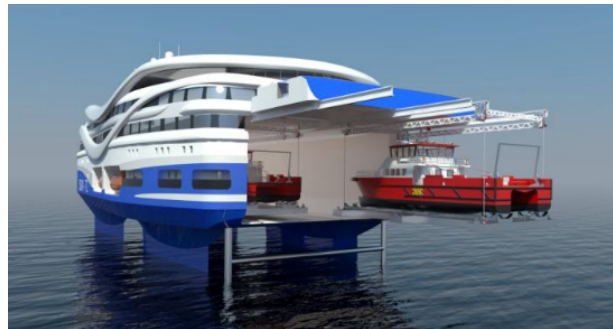
Figure 5.4: SOV alterations allowing increased dimensions for daughter crafts [McCartan et al., 2015]
