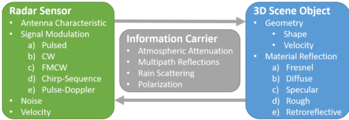
Figure 2.15: Physical structure of modeling radar sensor with reusable building blocks proposed by Thieling [27]
