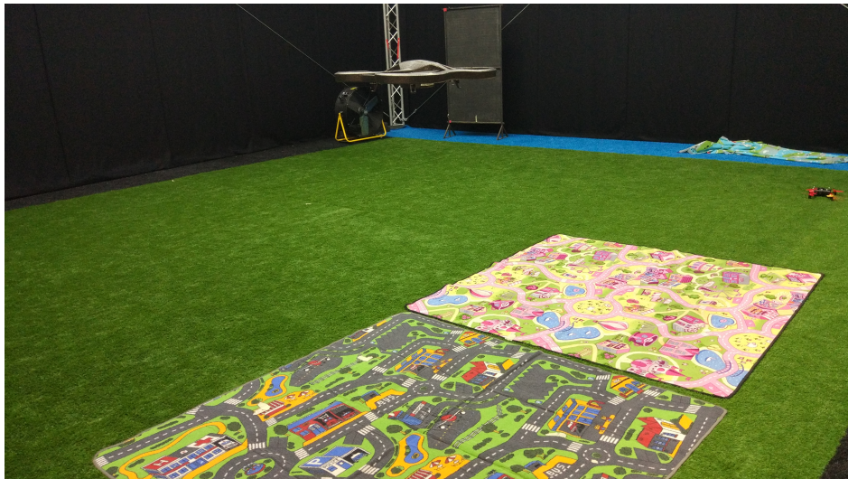
Figure 5-2: The ARDrone 2 flying in the Cyber Zoo, with play mats for additional features
