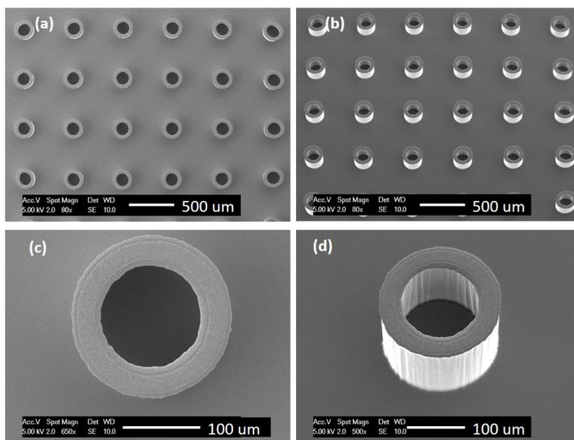
Figure 3.29: SEM images showing the fabrication results of hollow TPV structures with a inner diameter of 150  $\mu\text{m}$  and a wall thickness of 30  $\mu\text{m}$ . (a) Top view of TPV array. (b) Tilted (26°) view of TPV array. (c) Top view of a single TPV structure. (d) Tilted (26°) view of a single TPV structure showing clear inner wall surface and a clean inner bottom surface.
