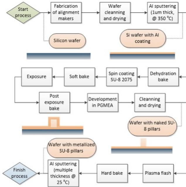
Figure 4.3: Process flow of the metalized TPVs samples used in the shear test.
