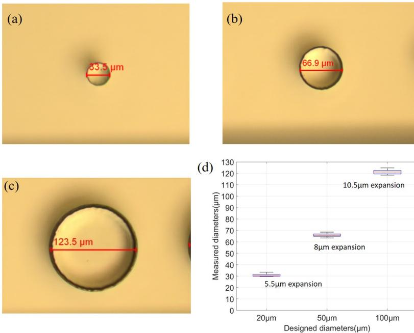
Figure 4.4: Measurement pillar diameters under optical microscope. (a-c) Examples of the measurement on TPVs with designed pillar diameters of 20  $\mu\text{m}$ , 50  $\mu\text{m}$ , and 100  $\mu\text{m}$ , respectively. (d) The measurement results of the distribution and average value of the pillar diameters over 6 process wafers and the calculated average expansion of the diameters.
