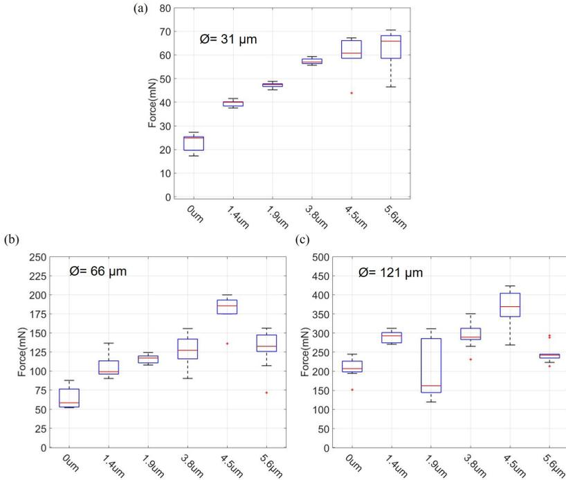
Figure 4.9: Boxplots of the distribution and average of the maximum shear forces of TPVs with different metal coating thicknesses. (a) TPVs with diameter of 31  $\mu\text{m}$ , (b) TPVs with diameter of 66  $\mu\text{m}$ , (c) TPVs with diameter of 121  $\mu\text{m}$ . The values of x axis ticks are the metal coating thickness
