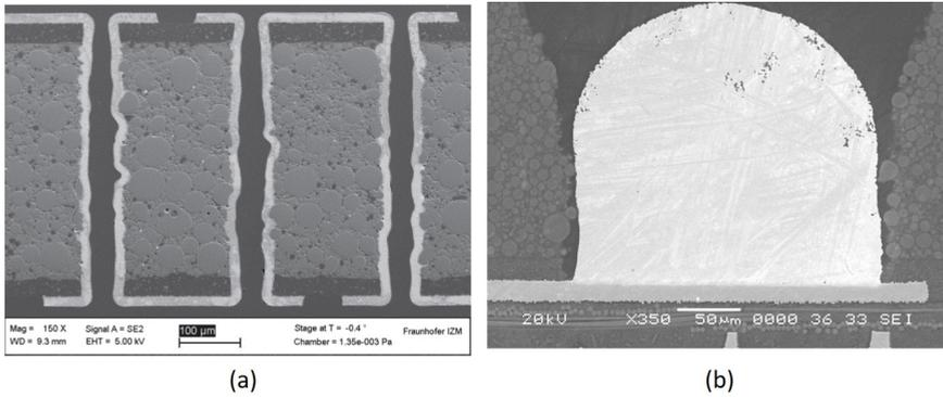
Figure 1.5: SEM images of TMVs. (a) TMVs with Cu coating, figure adapted from [15]. (b) A TMV filled with sold ball [7].
