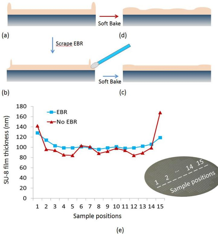
Figure 2.4: The comparison of film thickness uniformity with and without scrape EBR of the 100  $\mu\text{m}$  thick spin coating recipe on silicon wafers. (a) The edge bead builds up after the spin coating, (b) the process of scrape EBR, (c) soft-baking after scrape EBR, (d) soft-baking without EBR. (e) The measured film thickness with and without scrape EBR. The pitch between the sample positions is 6 mm and the diameter of the wafer is 100 mm.
