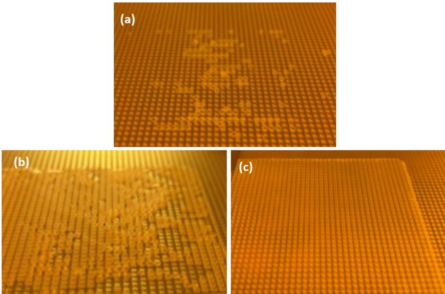
Figure 3.25: Adhesion improvement of the TPV ring structures. (a) Poor adhesion observed with strong over-exposure (340s at 10 mW/cm<sup>2</sup>) of SU-8 dry film and PEB at 95 °C. (b) Improved adhesion of the ring structures by PEB at 120 °C. (c) 100% adhesion of the ring structures achieved by PEB at 130 °C.
