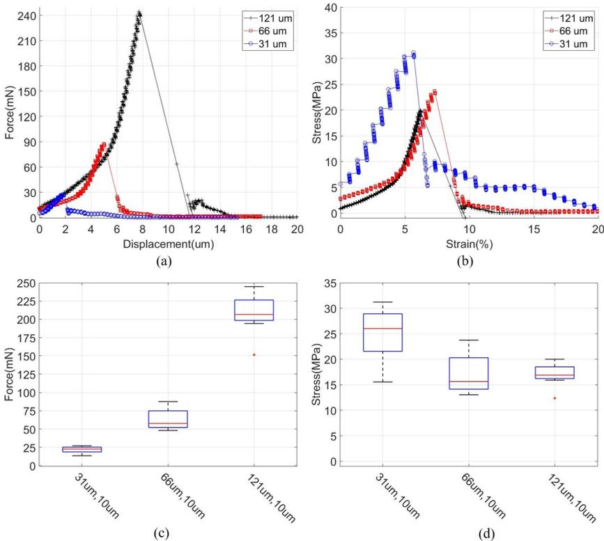
Figure 4.10: The influence of the pillar diameter to the shear strength of the uncoated TPVs. The shear height is 10  $\mu\text{m}$ . (a) The shear force against displacement, (b) the shear stress against strain, (c) the distribution and average of max. shear forces, (d) the distribution and average of max. shear stress. For the box plots, on the x-axis, the first dimension is the TPV diameter and the second dimension is the shear height
