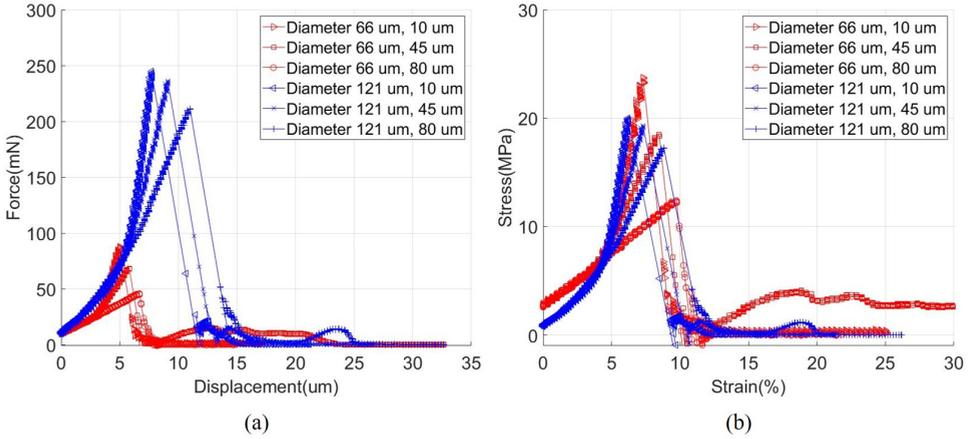
Figure 4.15: The influence of shear height to the shear response of the uncoated TPVs with diameter of 66  $\mu\text{m}$  and 121  $\mu\text{m}$ . (a) The shear response curve of force measured against displacement, (b) the calculated shear stress against strain.
