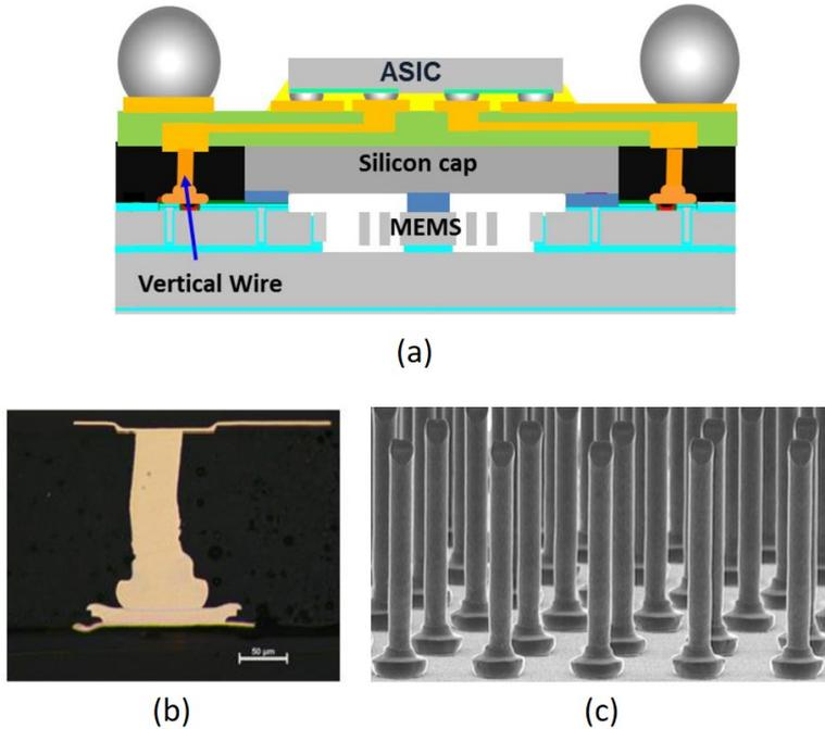
Figure 1.8: Through package vertical interconnection made of vertical wire bonds. (a) The application of vertical wire bonds in a MEMS WLCSPP packaging process. (b) The cross-sectional view of a vertical wire bond interconnection after molding. (c) The SEM image of high-aspect-ratio vertical wire bond array. Figures adapted from [8, 22, 35].
