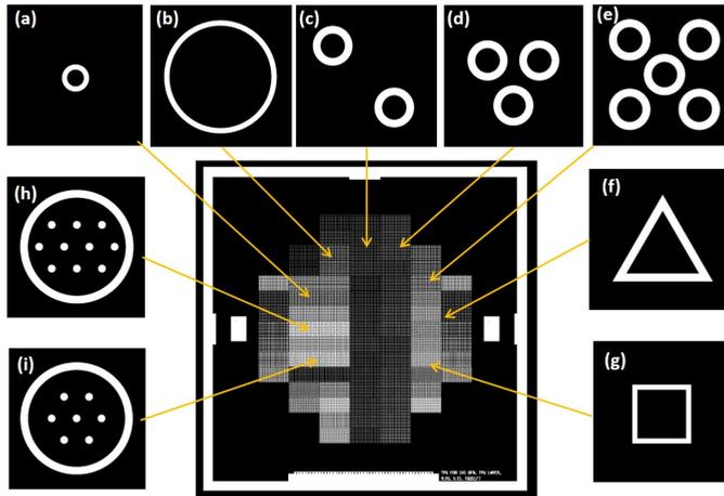
Figure 3.27: The mask design used in the TPVH-W-QFN process. (a-i) examples of the hollow TPV designs. (a) and (b) represents ring structures with a different inner diameter and wall thickness. (c-d) shows the design of making multiple structures on a single die area. (f) and (g) shows triangular and rectangular designs. (h) and (i) shows the design of structures which contains micro-pillars inside the through-hole.
