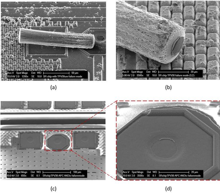
Figure 3.6: SEM images of delaminated TPVs and the delamination site on the contact pads. (a) A delaminated metallized TPV on the substrate. (b) The view of the delaminated pillar bottom. (c) The delamination site on the substrate. (d) Zoom-in view on the delamination site.
