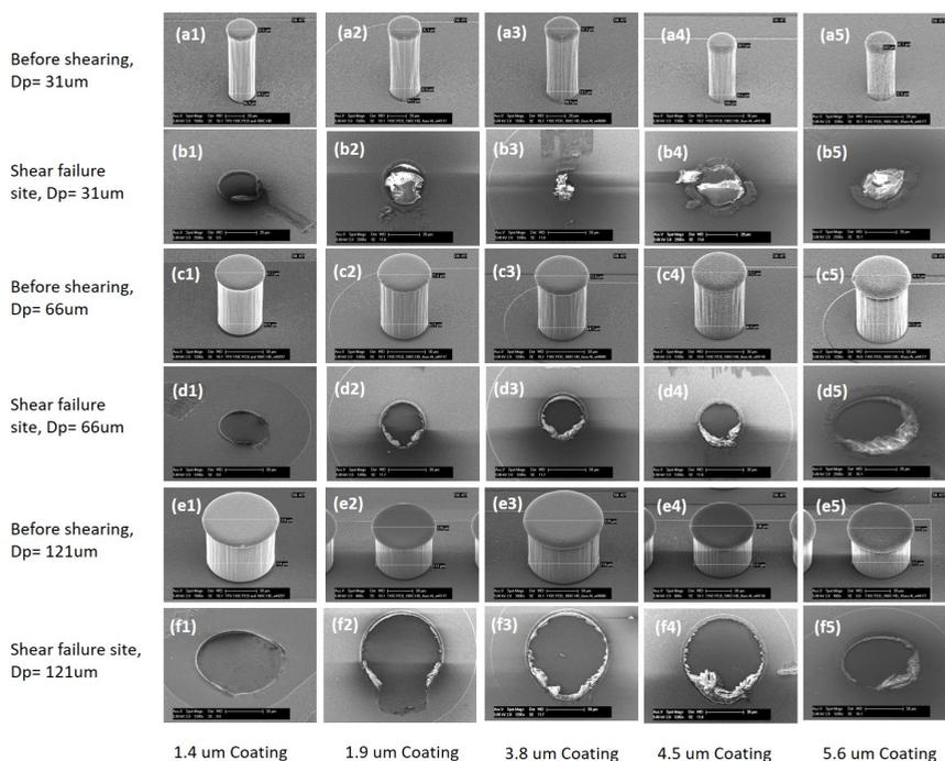
Figure 4.7: SEM images of metalized TPVs and their shear sites (the shear height is 10  $\mu\text{m}$ ). The fabricated metalized TPVs with different Al coating thicknesses with a diameter of 31  $\mu\text{m}$  (a1-a5), 66  $\mu\text{m}$  (c1-c5), and 121  $\mu\text{m}$  (e1-e5), and the shear sites of the metalized TPVs with different Al coating thicknesses with a diameter of 31  $\mu\text{m}$  (b1-b5), 66  $\mu\text{m}$  (d1-d5), and 121  $\mu\text{m}$  (f1-f5).
