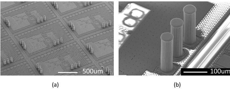
Figure 3.7: TPVs fabrication results from the optimized process setting. (a) TPVs on chip array, each chip has 20 GSG ports which requires 6 TPVs in total. (b) Close-up view of the optimized TPVs.
