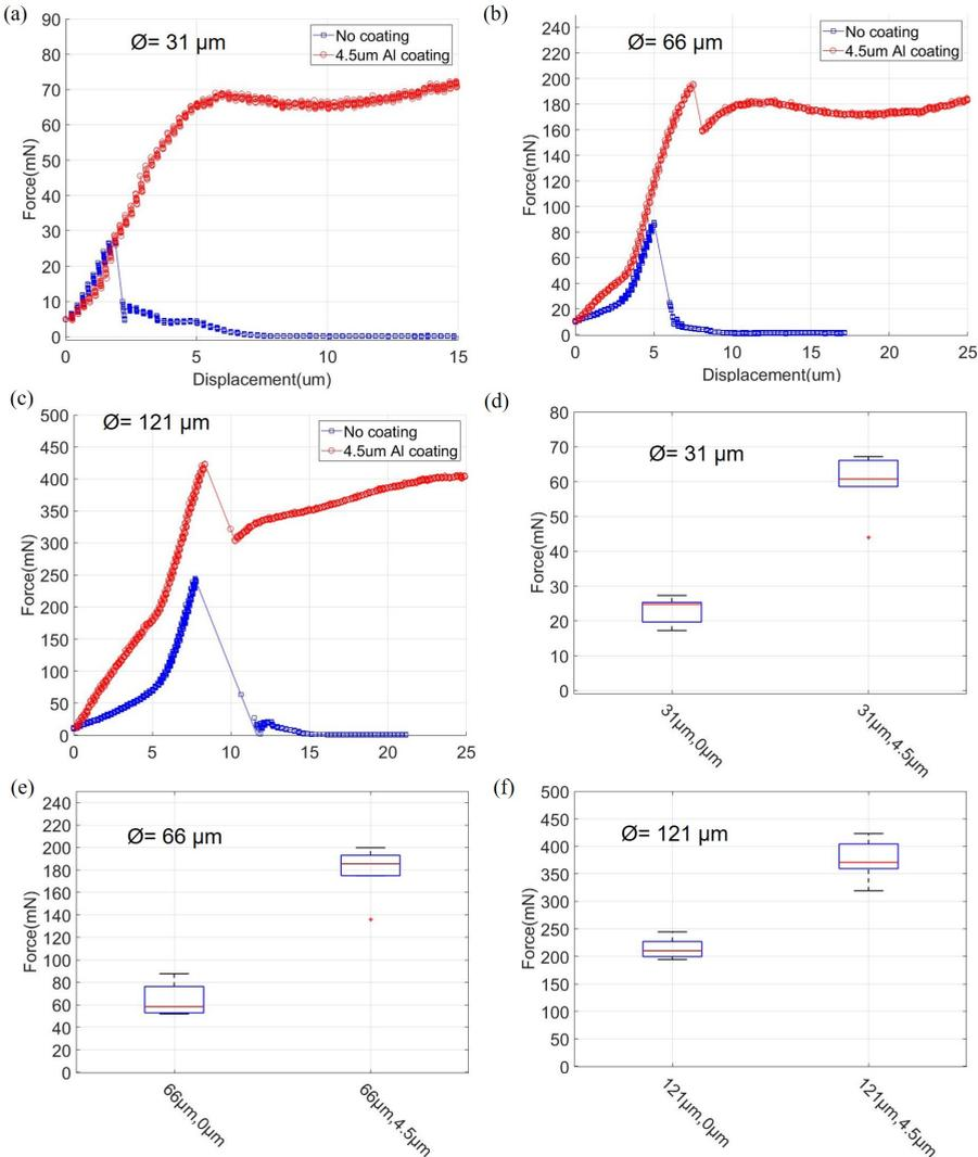
Figure 4.8: The comparison of the shear response of TPVs without coating and with 4.5  $\mu\text{m}$  thick Al (1%Si) coating. The pillar diameters are 31  $\mu\text{m}$ , 66  $\mu\text{m}$ , and 121  $\mu\text{m}$ . The shear height is 10  $\mu\text{m}$ . (a-c) The shear force response measured against displacement, (d-f) box plots showing the max shear force distribution over multiple measurements.
