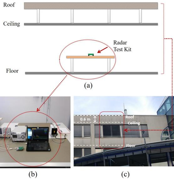
Figure 5.8: A schematic of the test environment. Both the ceiling and the roof of the building were used as targets. (a) Schematic illustration of the test environment, (b) the measurement setup including a laptop and the test kit, (c) photograph of the detected building features from outside.
