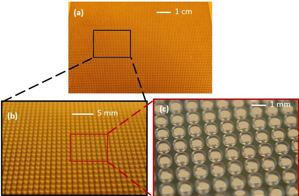
Figure 3.23: Fabrication result of TPV ring structures on PCB. (a) Overview of the entire PCB after TPV fabrication. (b) A good adhesion of SU-8 rings are achieved, no delamination is observed. (c) Close-up view of the SU-8 ring structures.
