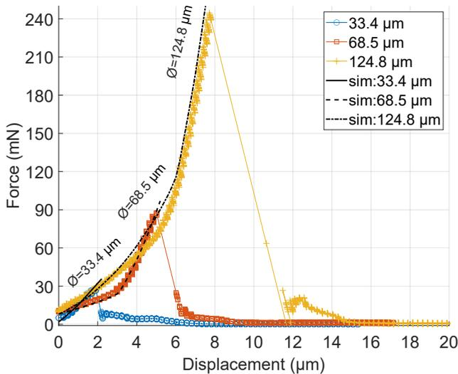
Figure 4.13: The comparison of the measurement and simulation results of the shear response of the uncoated pillars with diameters of 33.4, 68.5, 124.8  $\mu\text{m}$  at a shear height of 10  $\mu\text{m}$ .
