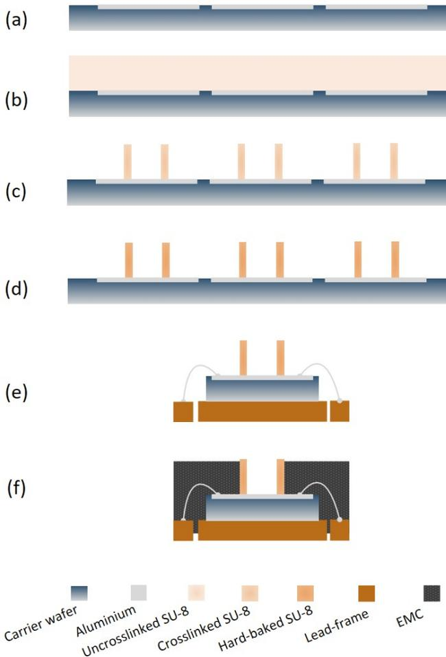
Figure 3.28: A detailed process flow of the TPVH-W-QFN process. (a) Al coating on bare silicon wafer. (b) Coating of thick SU-8 film. (c) The formation of hollow TPV structures. (d) Hard baking. (e) Assembly of the diced die to the QFN lead frame. (f) Film assisted molding.
