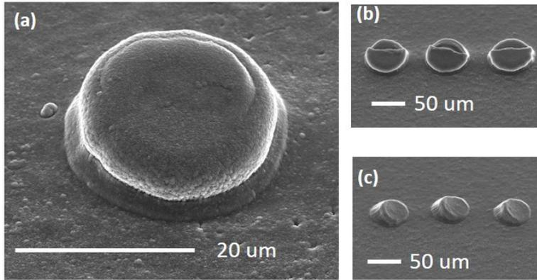
Figure 3.8: Protruding TPV heads metalized with  $4\ \mu\text{m}$  Al(1%Si). (a) A desired well-protected TPV head after film-assisted molding. (b) TPV heads with partially delaminated top metal layer. (c) Bended TPV heads.
