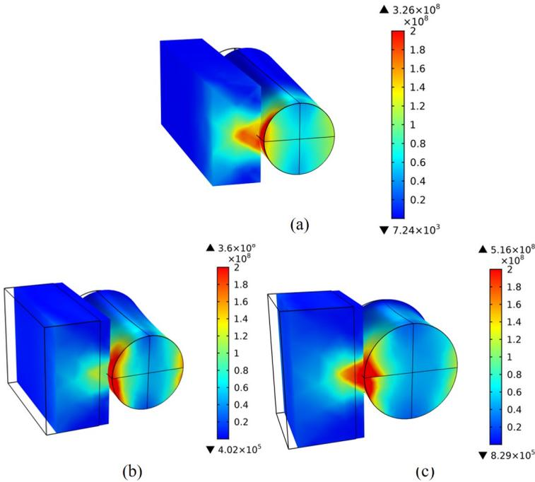
Figure 4.14: 3D simulation results of the stress distribution at the bottom of the SU-8 pillars at the failure points. The shear height is  $10 \mu\text{m}$ . (a) The bottom stress distribution of the SU-8 pillar with a diameter of  $33.4 \mu\text{m}$ , (b) the bottom stress distribution of the SU-8 pillar with a diameter of  $68.5 \mu\text{m}$ , (c) the bottom stress distribution of the SU-8 pillar with a diameter of  $124.8 \mu\text{m}$ .
