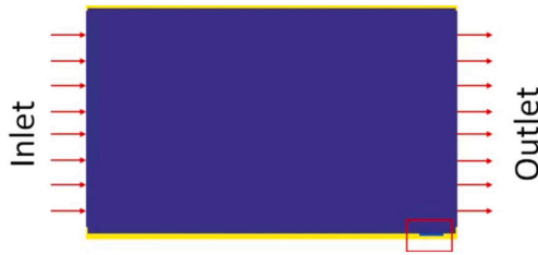
Fig. 5. Cross-section of simulation domain: mimicking the experiment setup in [11] with solution inlet, solution outlet and specimen (in the red box). (For interpretation of the references to colour in this figure legend, the reader is referred to the web version of this article.)
