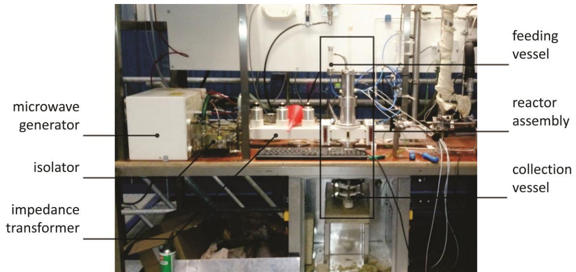
Figure 3. Photograph of setup with main parts indicated.
