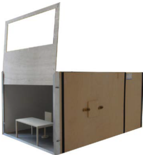
Figure 3.8: Image of scale-down model with removable window-side facade, adapted from [63]
