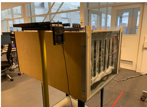
Figure 3.21: Test rig with reference cell on yellow pole mounted close to curtain
