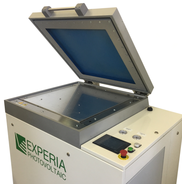
Figure C.2: Experia Photovoltaic LAM600 laminator used for laminating the mini modules in chapter 3
