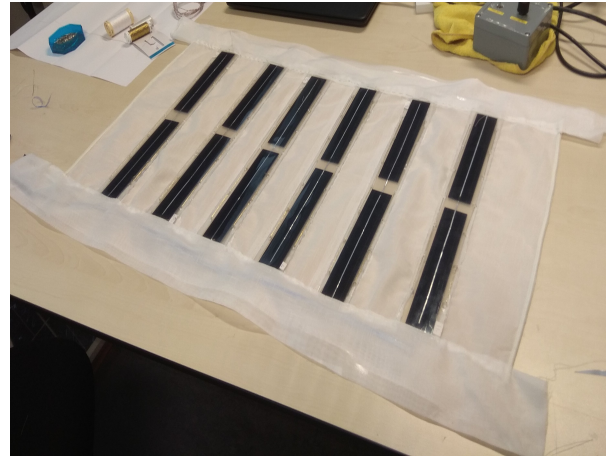
Figure 3.18: Tabbing wires between mini modules enclosed in cloth collars to make curtain module
