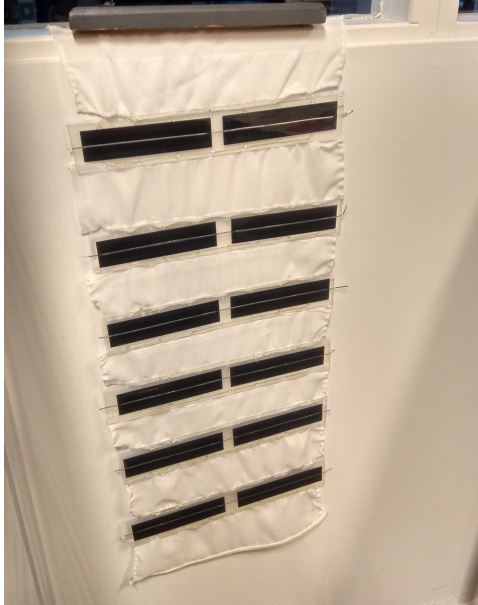
Figure 3.17: Intermediate stage of curtain fabrication after connecting cloth and PV strips
