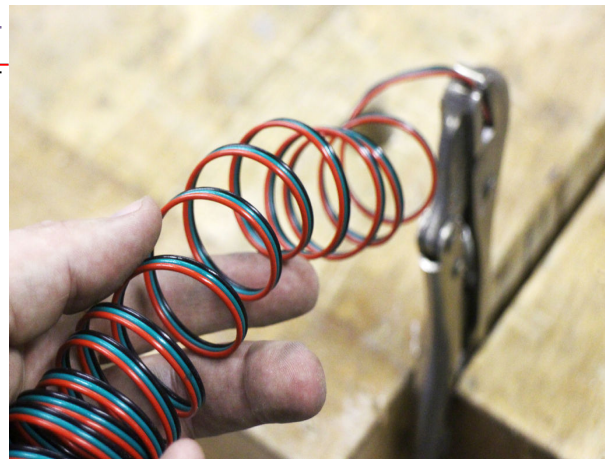
Figure 4.9: Coiled cables proposed for curtain connections [75]
