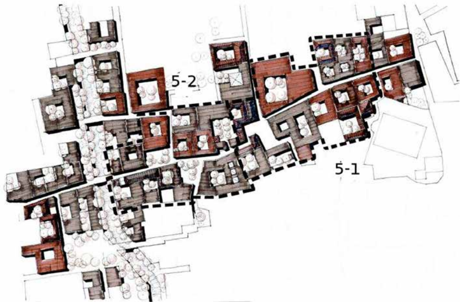
FIGURE 4.45 The schematic design of zone 5 produced by Bavand Consultancy. The historical houses are being reused to provide accommodation for cultural activities. A connecting passageway Passes through this zone and connects two main axis of the area (Persian Cultural axis and Pilgrimage axis). Source: (Bavand 2011, p. 73)
