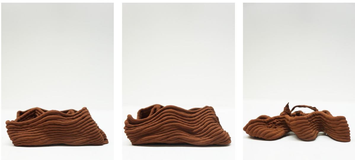
Figure 6.16: Overhang 20 degree with straight infill, Figure 6.17: Overhang 20 degree with zigzag infill, Figure 6.18: Overhang 20 degree olive shape
