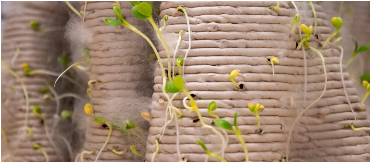
Figure 2.13: Urban Reef, 3D printing with mycelium and papier mache Source: https://www.urbanreef.nl/
