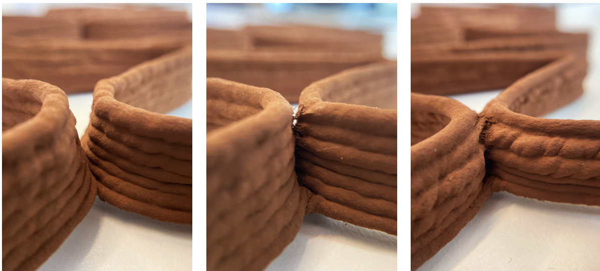
Figure 6.12: Printed 4mm overlap, Figure 6.13: Printed 2mm overlap, Figure 6.14: Printed 1mm overlap Source: own
