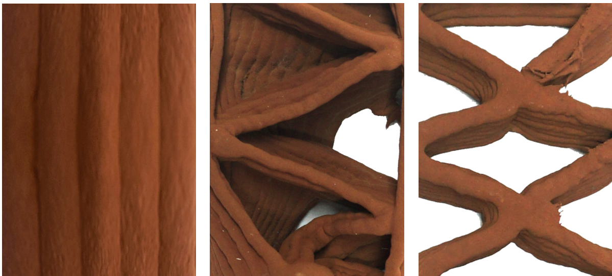
Figure 6.8: Printed 100% straight infill, Figure 6.9: Printed 50% straight infill, Figure 6.10: Printed 50% curved infill Source: own
