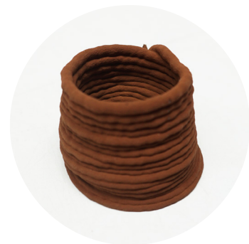
Figure 7.9: Maximum height limitation (safe height = 4cm) Source: own
