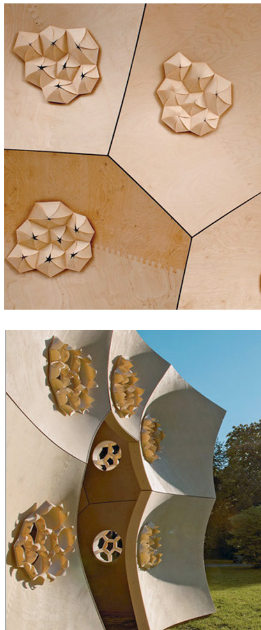
Figure 1.16. Hygroscopic shape-changing material Source: Materials in Progress : Innovations for Designers and Architects (2019)
