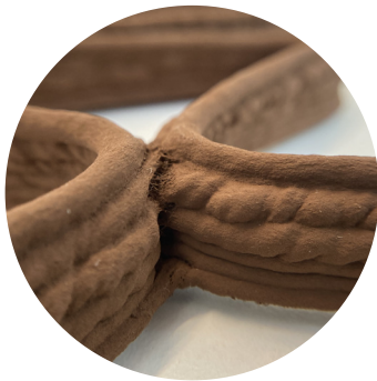
Figure 7.7: Overlapping between layers (1mm distance) Source: own
