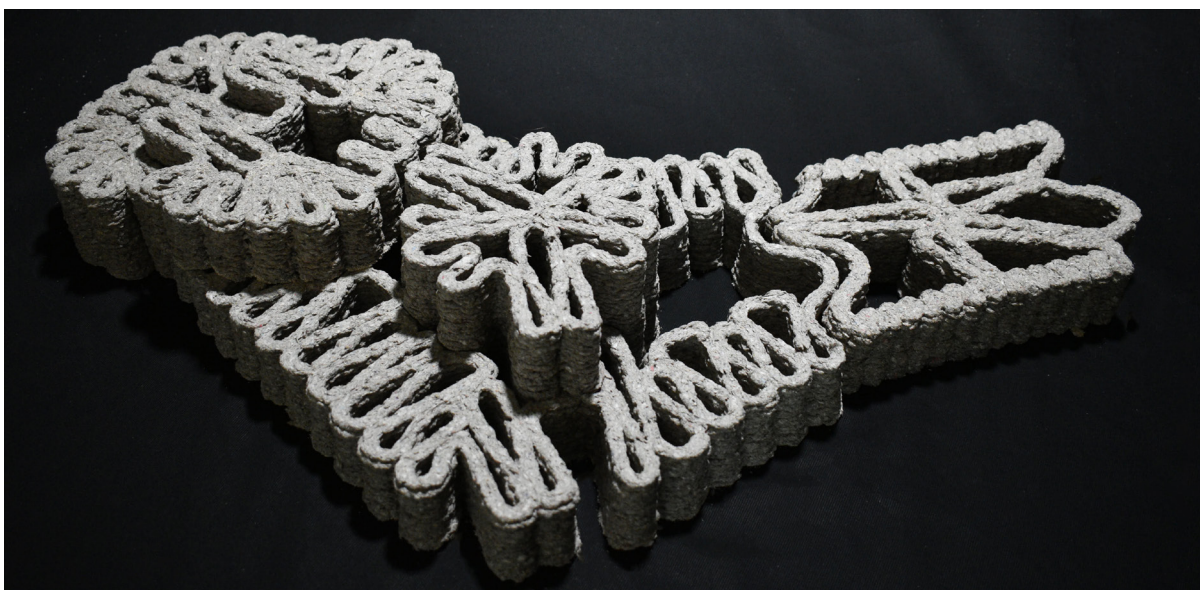
Figure 2.11: CITA, 3D printing cellulose based biopolymers
