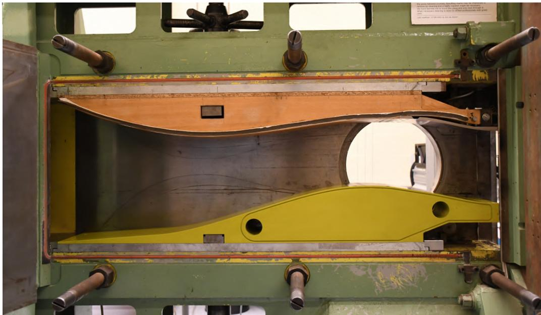
(b) Upper and lower test section blocks assembled in the ST-15 wind tunnel.
