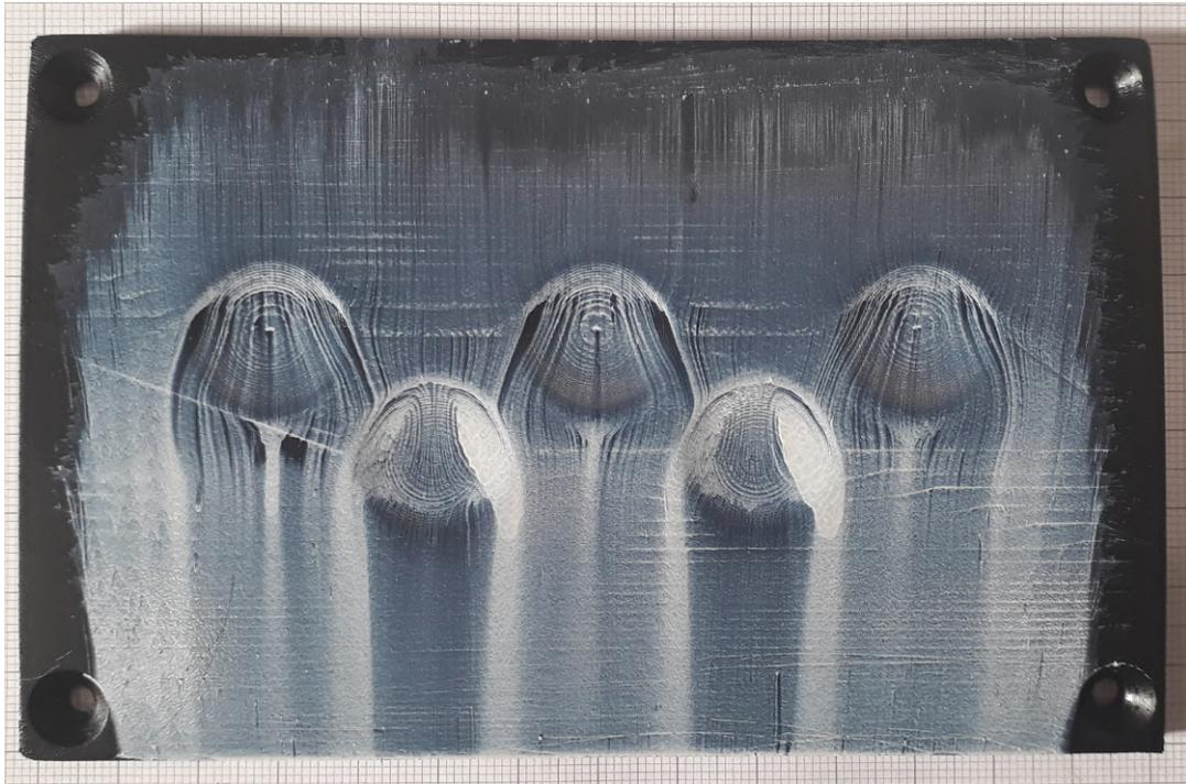
Figure B.7: Oil flow visualisation over the test plate covered with 1mm deep dimples (flow from top to bottom of the image).
