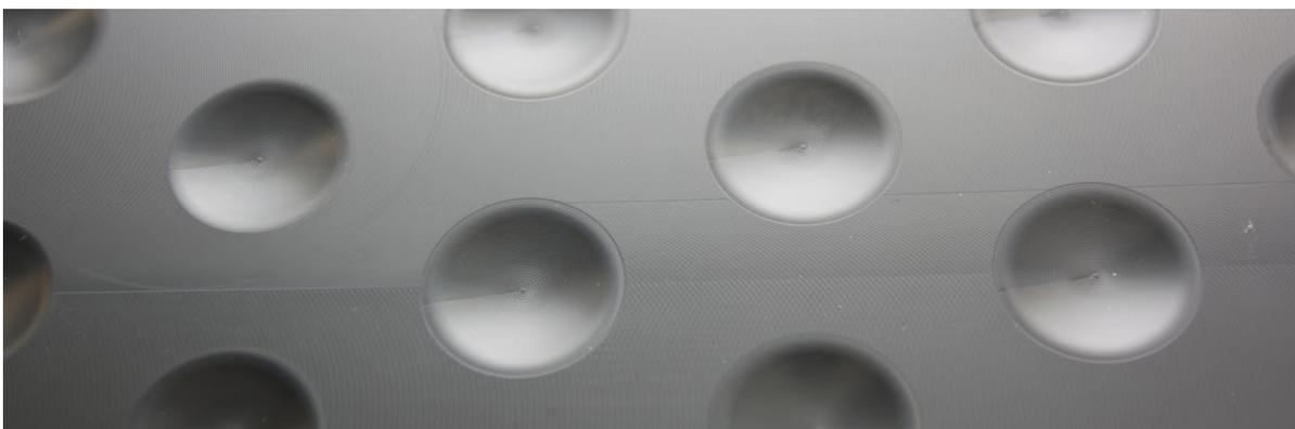
Figure 1.4: Example of a dimpled surface used to reduce viscous drag [93].
