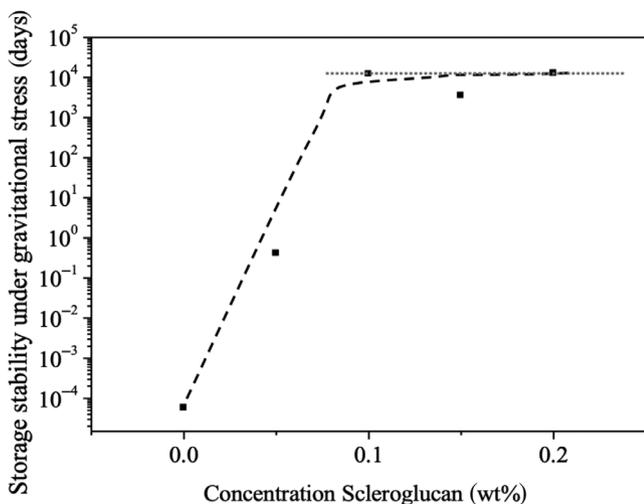
**FIGURE 3** Delay time under gravitational stress in function of the scleroglucan concentration. Note the time scale is in days, not seconds
