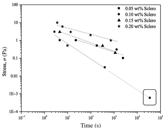
**FIGURE 2** Stress as a function of the delay time. ■ 0.05 wt% scleroglucan, • 0.10 wt% scleroglucan, ▲ 0.15 wt% scleroglucan, and ★ 0.20 wt% scleroglucan. A power law regression is used to extrapolate to the stress exerted by gravitational forces. The data point inside the square for 0.05 wt% is the estimated delay time calculated using Equation (1) and is also plotted in Figure 3
