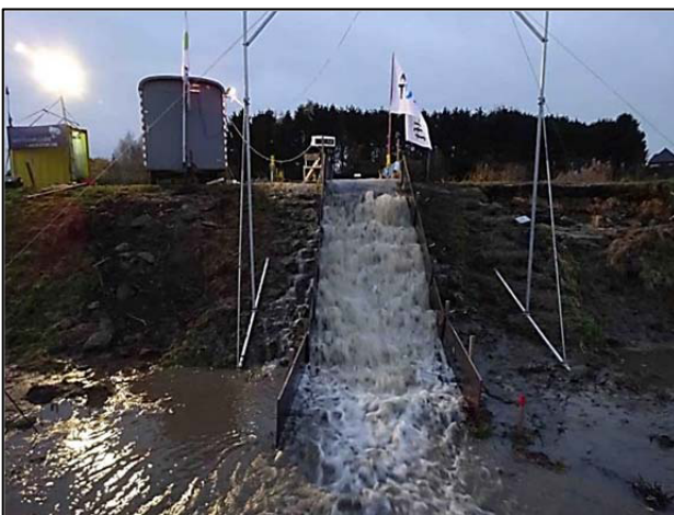
Figure 6. Observed aerated flow during the overflow experiment
