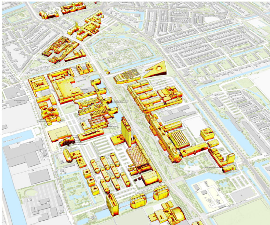
Figure 23. Annual solar irradiation map for TU Delft campus. Through this link https://tudelft.maps.arcgis.com/home/webscene/viewer.html?webscene=0bc9d9485c334a07aa05402238776477 , one can see all the simulation results by logging in with a personal Google account.
