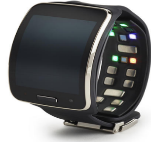
Figure 5.1: The Samsung Simband 2 with multiple channels for ECG and PPG. Source: [21].
