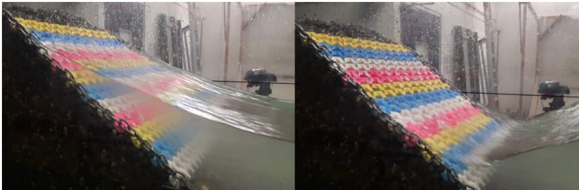
Figure 5.10: Left: wave crest induces high core water level, right: wave through induces outward directed pressures by water wanting to flow out
