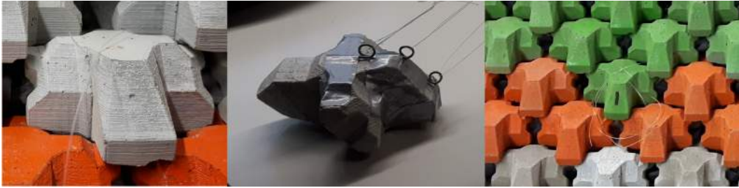
Figure 4.2: Methods of securing fishing line: "Simple", "3 loops" and "Cross"
