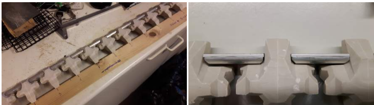
(a) Distance between units is exactly 1.1 \cdot D_{n50}
