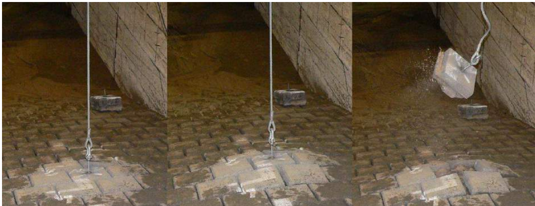
Figure 2.13: Full-scale pull-out test on Verkalit interlocking placed block, chronological sequence [Gier et al., 2012]
