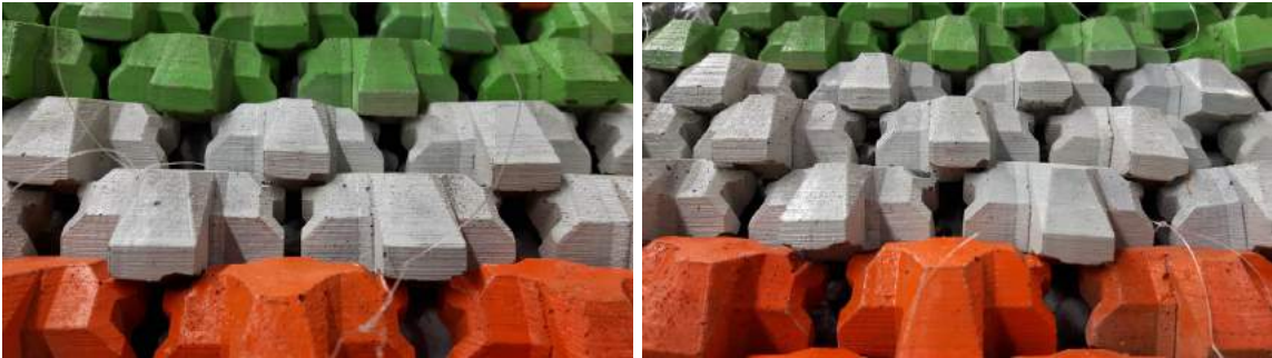
(a) Only chamfers make contact (b) Nose supported on one side only
