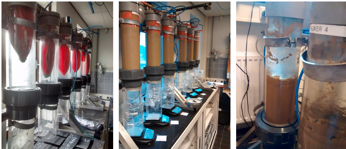
Figure 5.1: Experimental consolidation and discharge capacity test: (left) sample tubes with loading balloon, (middle) consolidation tests without drains, (right) permeability test on a consolidated sample with a drain.
