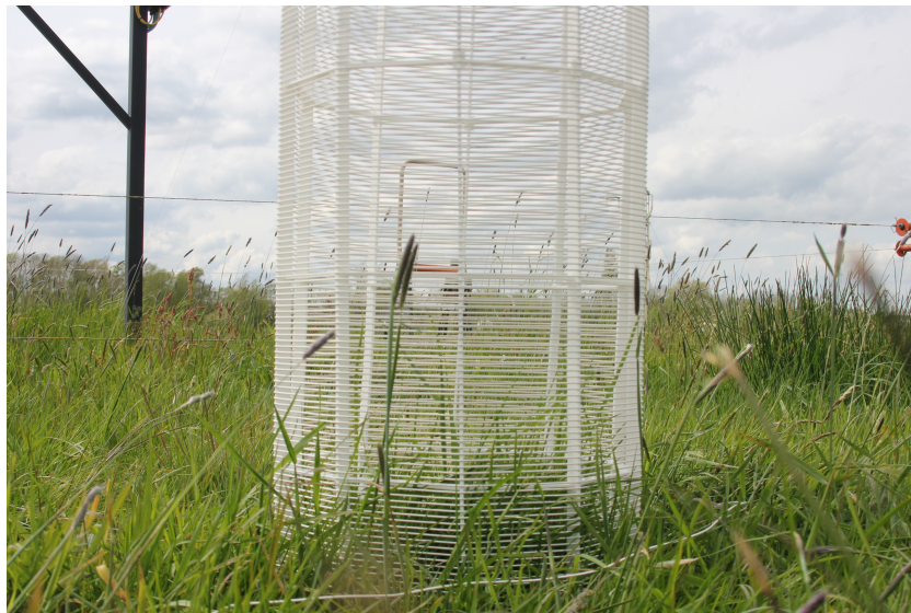
Figure 6.3: The DTS coil at Cabauw with the grass field where the measurements were executed. Note that the grass is not uniform in height.
