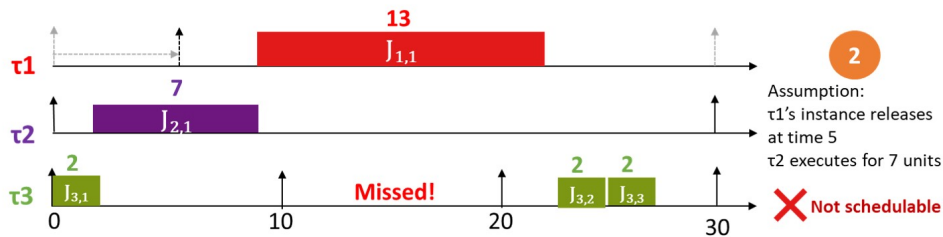
(c) Schedule where \tau_1 releases at time 5 and \tau_2 executes for 7 units
