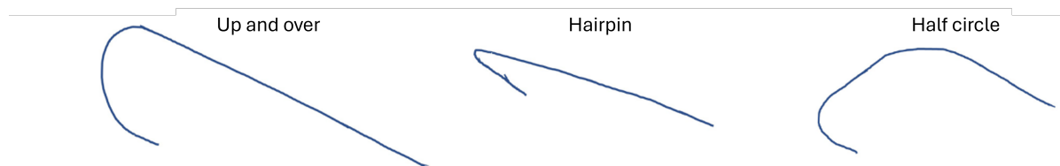
Figure 1.1.4: Trajectory of the Front Wheel Hub During BMX Start. The figure displays the path of the front wheel hub during the start. BMX rider moves from left to right. Adapted from Grigg [13].
