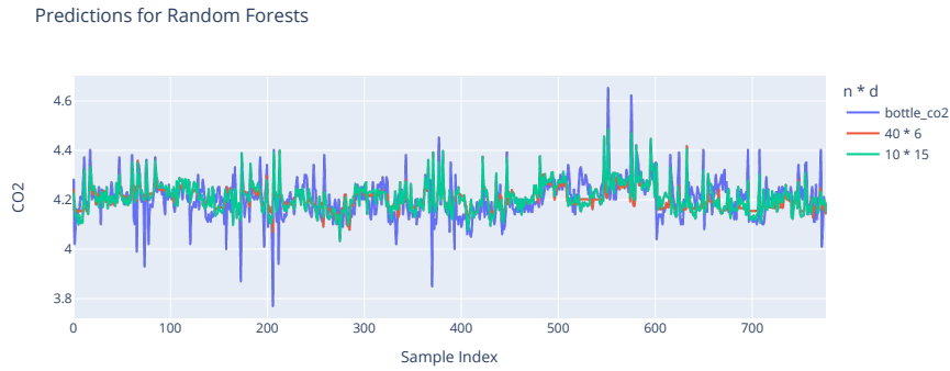
Figure 6.11: Predictions on all test set samples using two random forests for comparison. The first with 40 trees of depth 6 obtained a MAE of 0.0040, while the second with 10 trees of depth 15 achieved a MAE of 0.0044.
