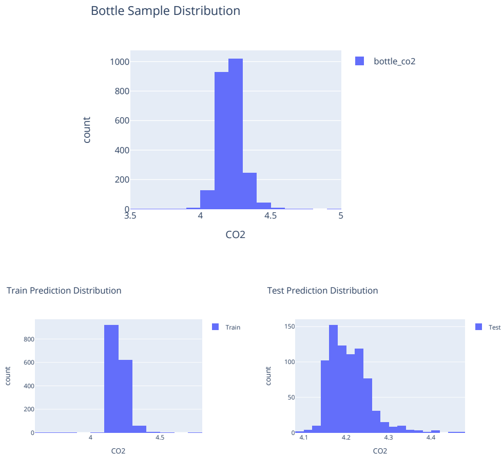
Figure 6.10: Distributions for the entire dataset and predictions on the train and test set, demonstrating that the model does not merely output the general mean of the target values.
