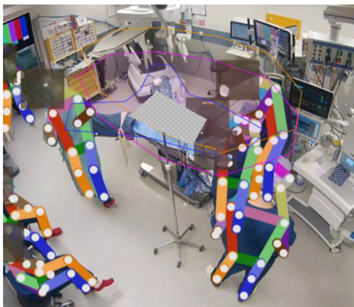
Figure 22: Screenshot from a video recording showing various zones around the operating table. The blue, purple, and orange lines, are all considered in deriving the Interaction with Operating Table Score.
