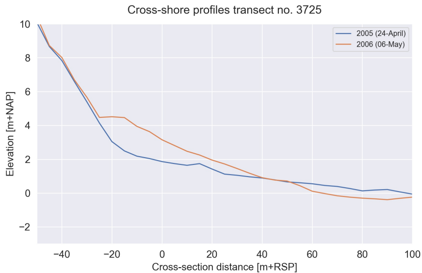
Figure 4.14: Two JARKUS cross-shore profiles are depicted of an arbitrary transect, where distinctive features of the beach nourishment (performed 2005) are indicated in the cross-shore profile of 2006.
