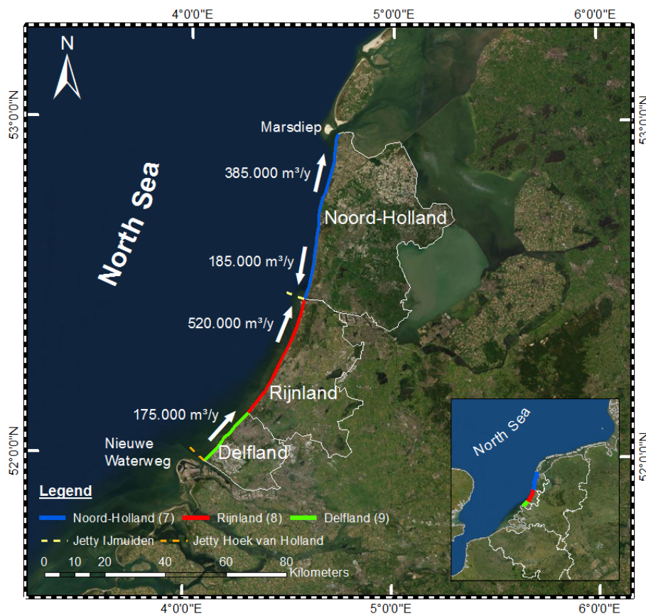
Figure 3.1: An overview map of the central Holland coast with the coastal sections (Noord-Holland, Rijnland, and Delfland) and the corresponding longshore transports (white arrows). Be aware that the jetties are not drawn to scale. Source of longshore transport: Van Rijn (1995) .
