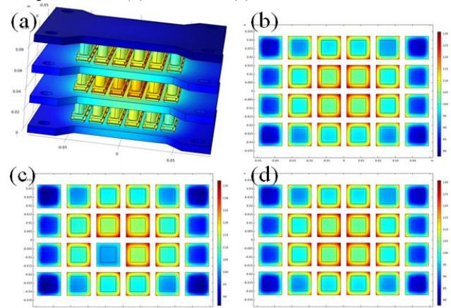
**Figure 4.** The thermal distribution of (a) the proposed IGBT module, (b) first subunit, (c) second subunit, and (d) third subunit.
