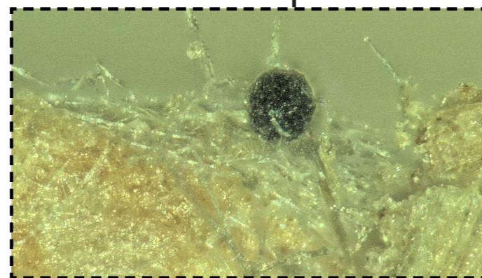
Surface | Local black spot | 400x magnification
