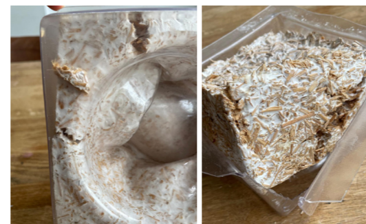
Broken sample because deformation of the mould
