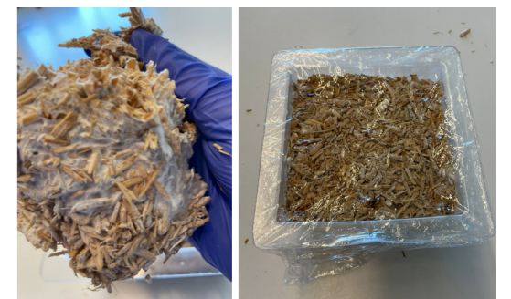
Left: The material had already begun to grow together; Right: Plastic foil with holes over the material.
