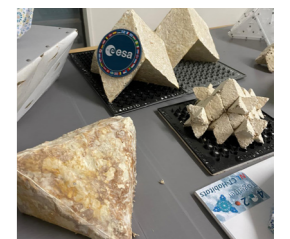
Optimal sized and formed brick to use in space.
