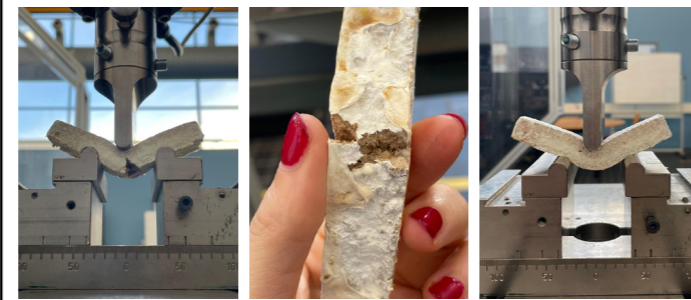
Maximum 25N for 9,5 mm deformation
