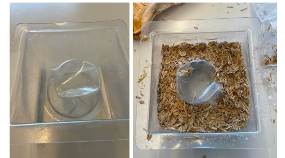
Deformation of the mould
