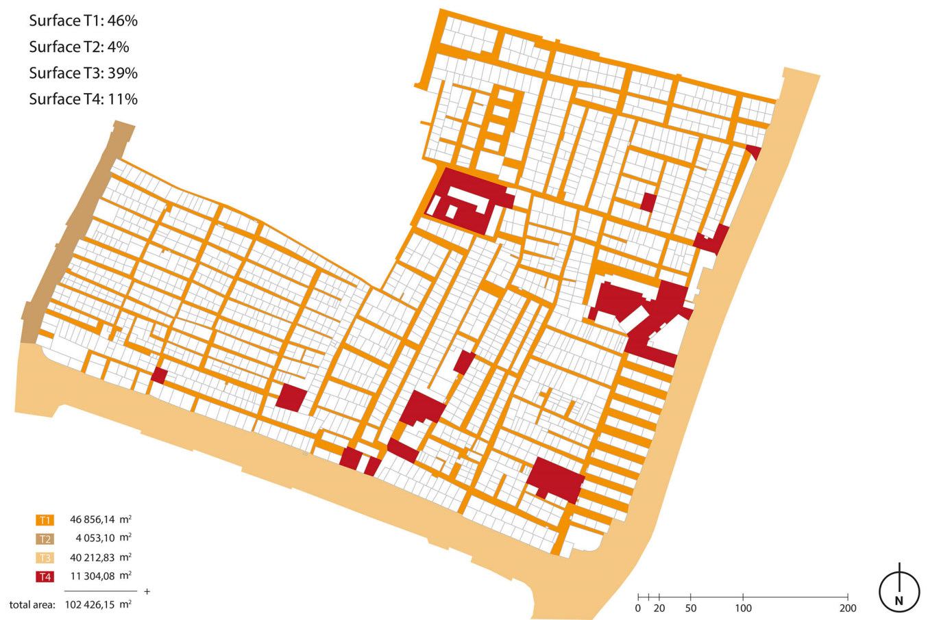
FIGURE 3 Spatial overview of the representative street typologies T1–T4 identified, and their distribution within the Shubra district. “T” stands for typology.
