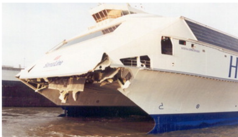
(a) Structural damage due to wetdeck slamming on HSS Stena Discovery during operations in the North Sea, in 1997
