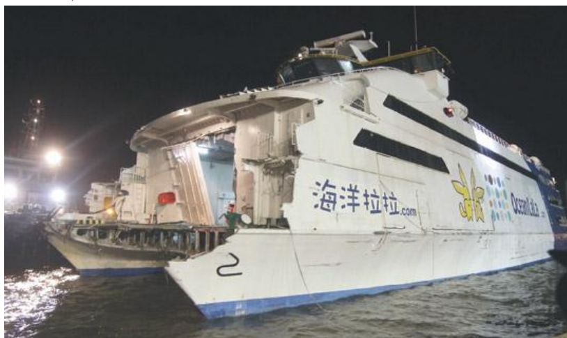
(b) Practical bow loss due to sever slamming on Ocean Lala during voyage from Penghy, Taiwan to Taichung, Chine, on August 2010
