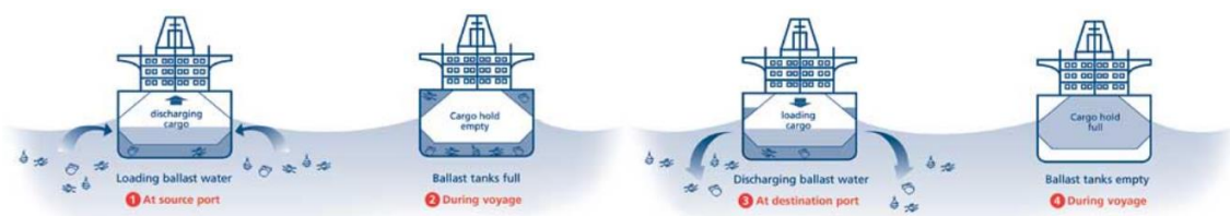
Figure 8 Procedure of release of ballast water (International Maritime Organization, 2017)
