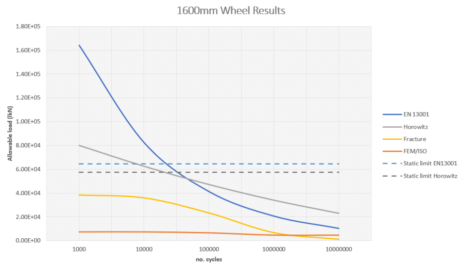
Figure 5.1: Results for all methods plotted for the 1600 mm wheel with static limits included
