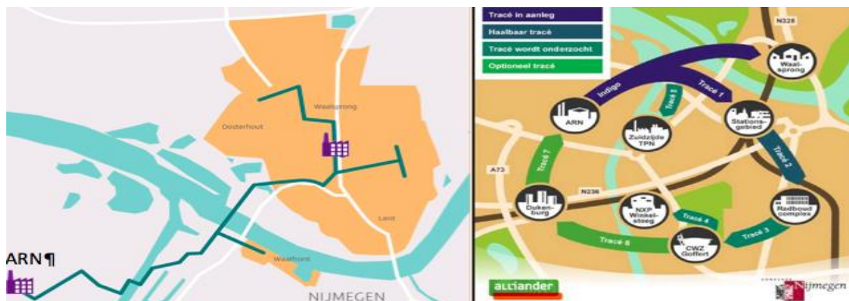
Figure 12. (l) The map shows the existing network for district heating in Nijmegen, with the waste power plant (ARN) as the source and the auxiliary heat plant Pieter Wiersma for peak hours (Nuon, 2016). (r) The map shows the planned extension of the district heating network (Liander, 2014).
