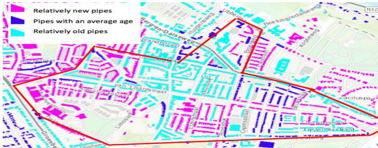
Figure 11. The online gas map provided by Liander, shows the age of the gas network in Hengstdal. New pipes are pink, older pipes are light blue. The dark blue buildings are pipes of average age (Liander, 2018).
