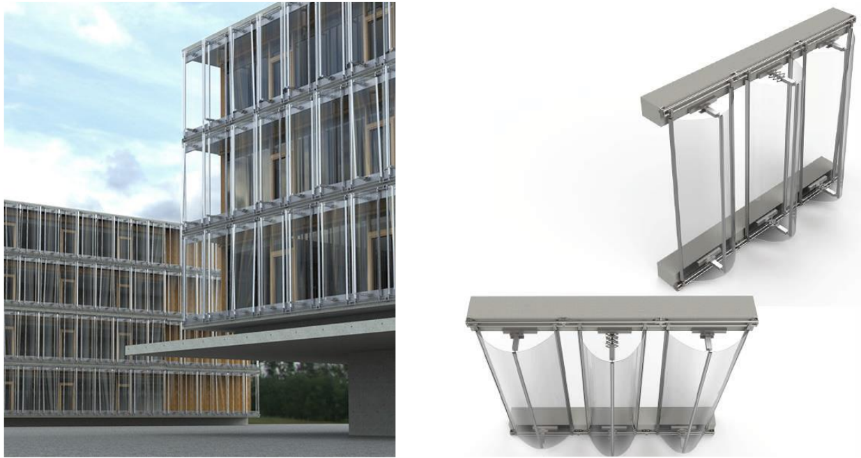
Figure 1.6 Adaptive thin Glass façade (Silveira, 2016)
