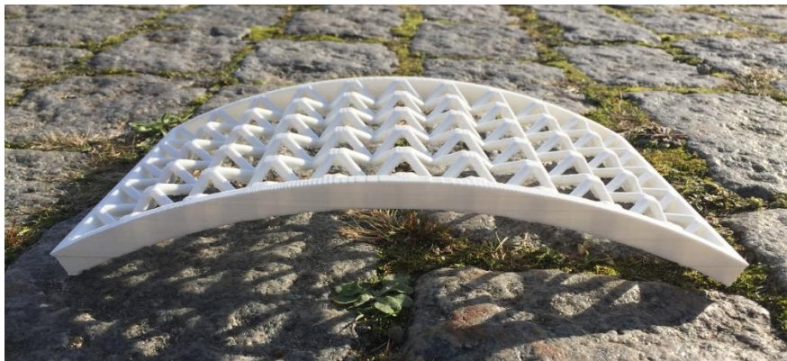
Figure 6.5 Curved truss core – FDM printed - Second trial - Side view
