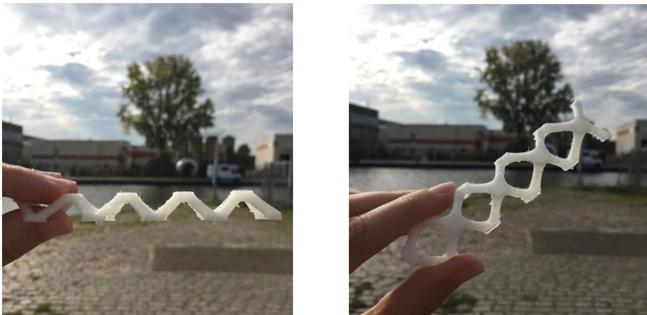
Figure 6.3 Truss core divided into straight strips
