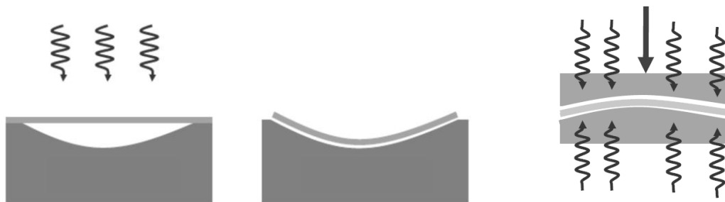
Figure 2.13 Hot Bending - Sag bending technique (left) and Autoclave (right) - (Louter, Material Characteristics, Production, Processing & Products, 2017)
