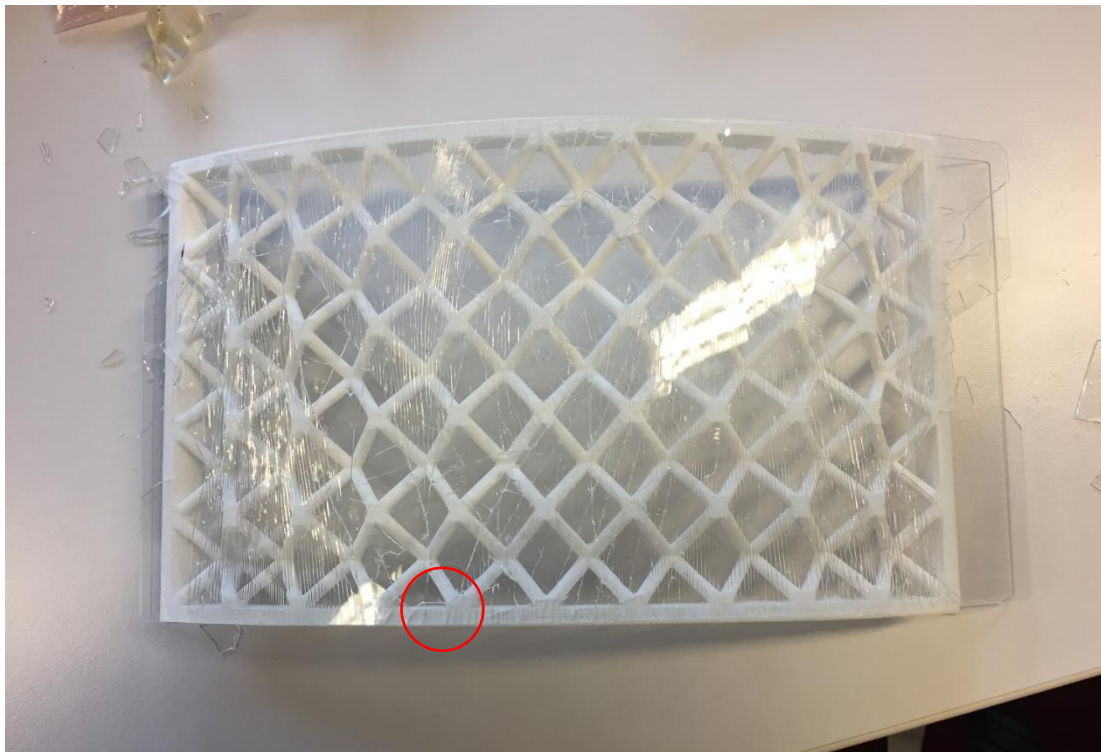
Figure 7.3 Panel 1.1 - Broken Top Layer of Glass
