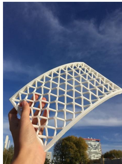
Figure 6.6 Curved truss core - FDM printed - Second trial - Perspective view
