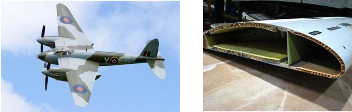
Figure 3.3 Mosquito aircraft (left), sandwich structure of an airplane wing (right)
