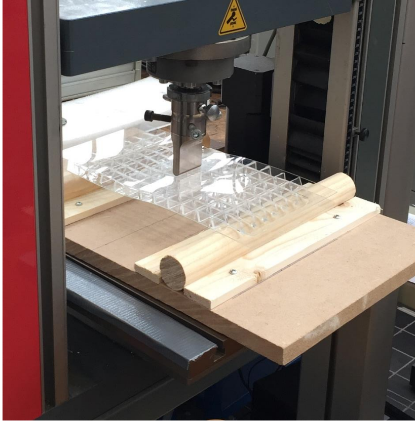
Figure 8.12 Deflection of Panel 2.1 during Testing
