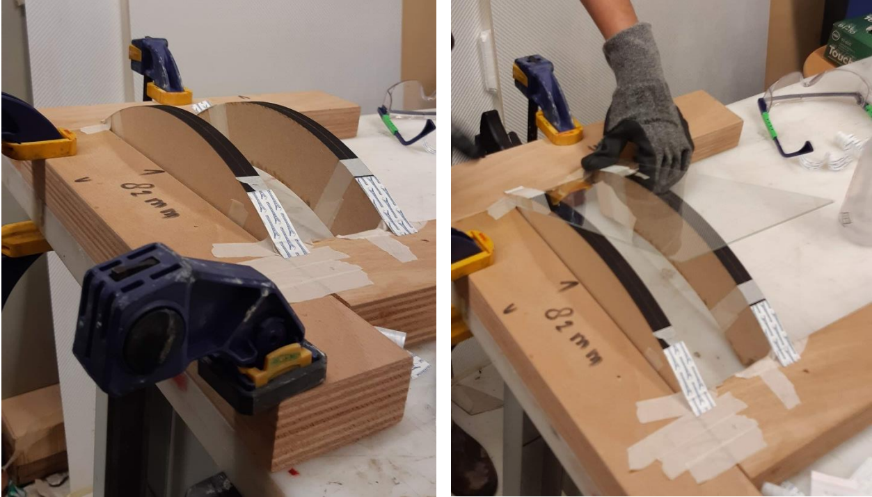
Figure 6.15 Wooden Mould to cold bent the glass
