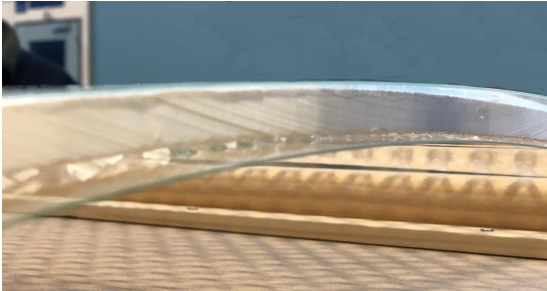
Figure 8.14 The Glue was already detached before start testing
