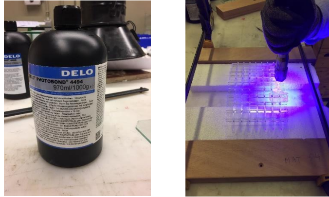
Figure 6.11 Delo Photobond 4494 acrylic glue cured with UV light
