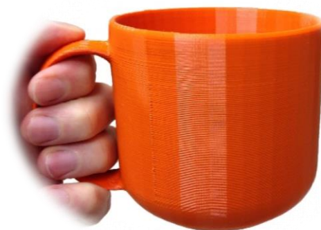
Figure 4.4 Fused Deposition Modelling (FDM) Product
