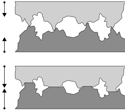
Figure 2.10: Contact asperity of steel surfaces [51]
