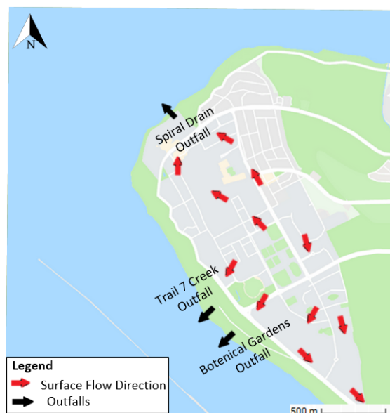
Figure 2.4: Stormwater Outfalls and the surface flow directions [10].
