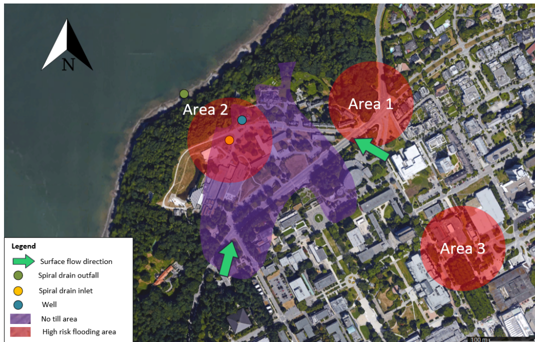
Figure 10.3: Project location with areas of greatest flood risk, the no till area, the spiral drain and drainage wells and the surface flow direction. Information from [54].
